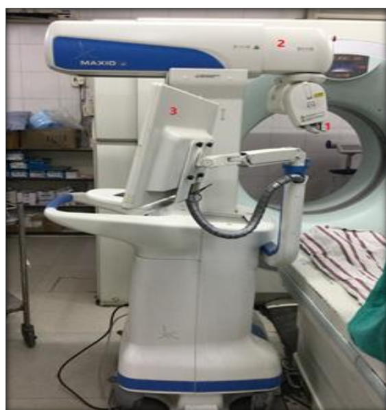
Figure 1: Showing the robotic system deployed in the study with its individual components viz (1) grippers (2) electromagnetic arm and (3) control panel
